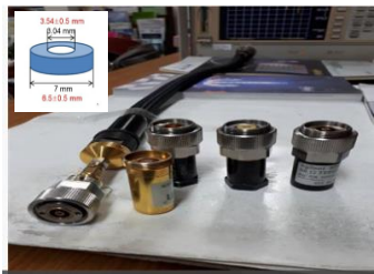
Sample Holder test set-up
