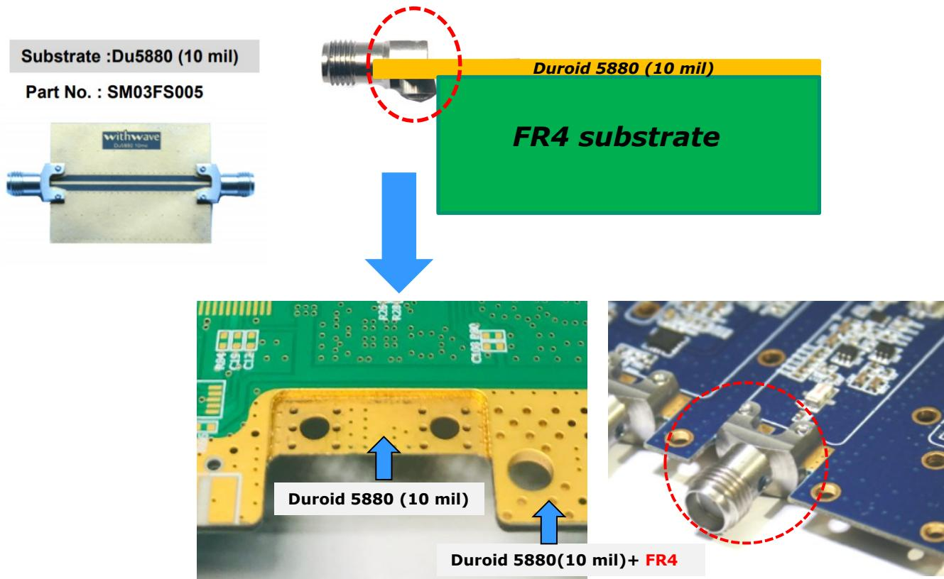
2. The edge of substrate should be contacted to body of connector directly. zero gap between substrate and body of connector is important to get good performance at the range of high frequency.
