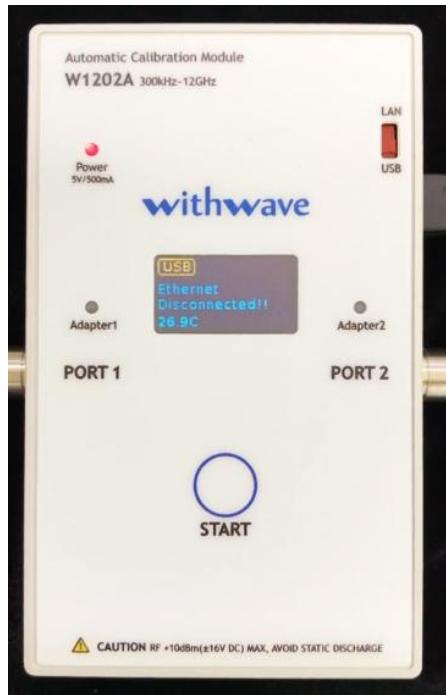
If USB ethernet connected successfully, OLED show "Ready for Calibration" message. and turn on **START button** led as shown picture below.
