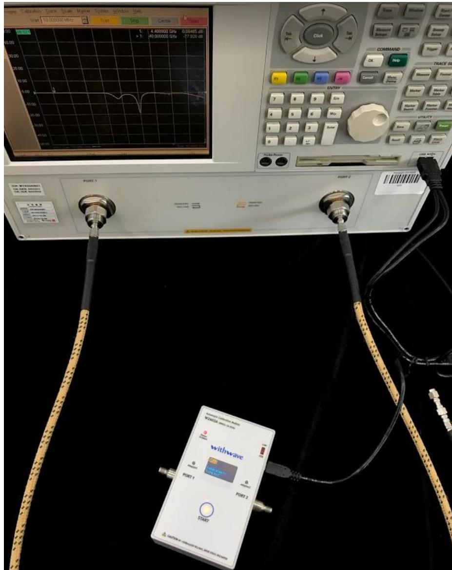
WACM will start system boot sequence if USB connected to VNA and it will take about 35 seconds.
